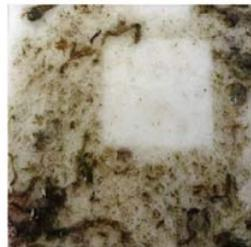
Evaluation of biofouling behaviour by marine immersion for 14 weeks (Baltic Sea, Germany) and investigation of the fouling-release properties by high-pressure water-blaster treatment (a common used method for ship cleaning).
